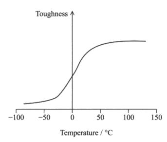
The brittleness and malleability of the steel also vary with temperature.
